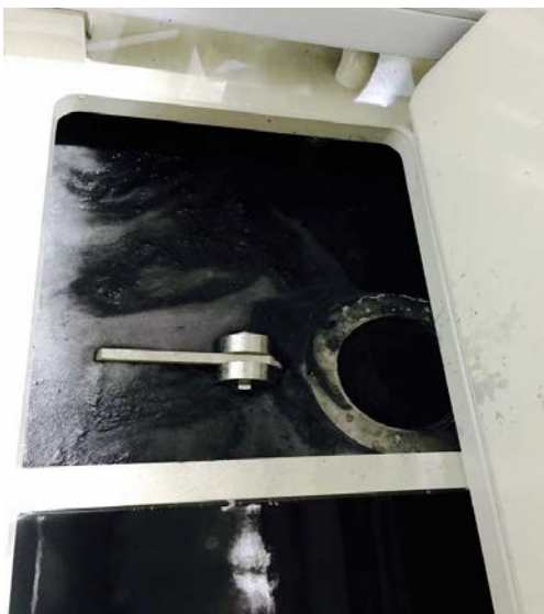
FLOATING SKIMMER WITHIN A DEGREASING TANK
