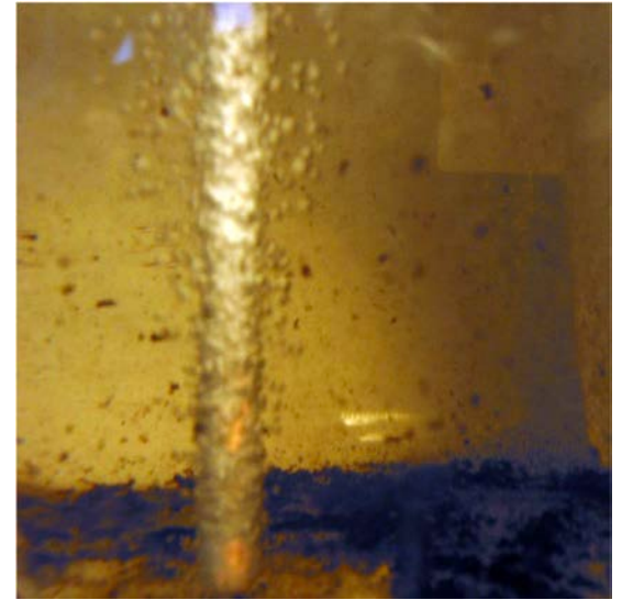
Gas bubbles generated by ultrasound on a wire surface
